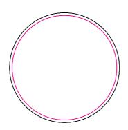
Print area is 40mm diameter Print position has a 2mm tolerance Magnenta line does not print!
